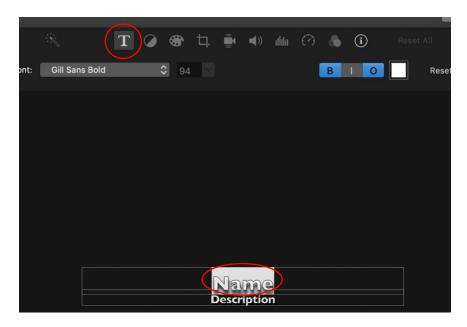
In the Description portion type the caption, keeping the length within one line of text. To change the style, select the Font: upper left drop-down menu. Scroll to the bottom to Show Fonts...
